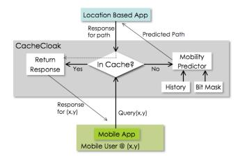
18: The system diagram for the centralized form of *CacheCloak*. Mobility prediction based on historical mobility patterns and the bit-mask of caches is performed at the intermediate server. LBS responses for the entire path is cached, and the responses forwarded according to the current (x,y) coordinate of the mobile user.
