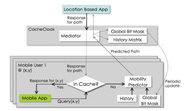
19: A distributed form of *Cache Cloak*. The historical patterns and the global bit-mask is periodically shared with the mobile device, which can then predict its mobility and request information along the predicted path. The path-wide responses are cached on the mobile. The Cache Cloak server is only necessary to maintain the global bit-mask from all users in the system.
